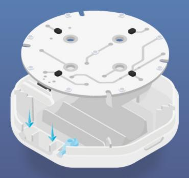
Line up the button with the groove in the base
